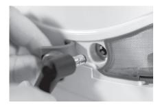
Connect one end of the AC power cord to the inlet on the power supply brick. Connect the other end to a wall outlet.
